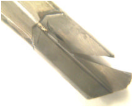
Fig. 3. Drill failure as a result of excessive misalignment.
