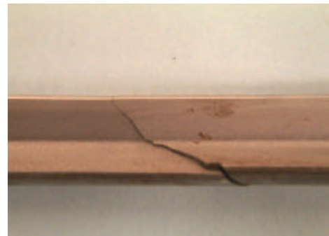
Fig. 4. Fatigue failure of the shank
